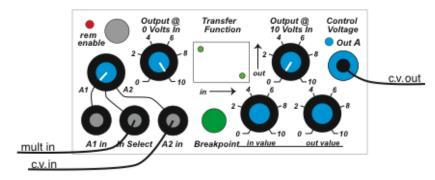
Now add a break point, such that the output stays at a constant 2 volts until the average of two inputs exceeds 8 volts – then the output voltage rapidly goes to 10 volts:
