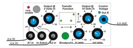
Here we use a voltage to control the proportions of two inputs that are applied to the transform matrix. The output starts at 8 volts, for an applied input of 0 volts, has a negative peak of 0 volts when the input reaches 2 volts, and then goes to 10 volts as the input reaches 10 volts:
