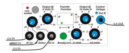
Note that the low resolution display provides a rough but useful indication of the transfer function. The actual voltages are calculated to a high degree of precision, and are appropriate for application to pitch and other variables.
