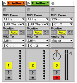
The example to the left shows the card being used to send Ableton MIDI clips to the Internal MIDI bus A and C as well as recording Internal MIDI bus B.
